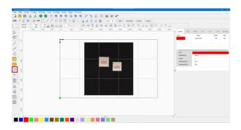
3. Set the processing method and processing parameters for each graphic, change the graphic positioning position in the lower right corner of the interface to "Absolute coordinates", select both "Output selected graphic" and "Selected graphic positioning", select the processing graphic, and download the file to the machine click [Start] on the machine operate panel to complete multi-position fixed processing.
