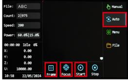
Please always remember to close the top lid and push the drawer in before: Click the start processing. Otherwise, the machine will not start working properly. Note: For more panel button functions, please refer to «How to use the operate panel» on the page 40.
