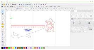
3. Set different color blocks for different processing techniques to distinguish the graphics. Click to select the corresponding graphics, move the mouse to the color block bar and select the corresponding setting and color.
